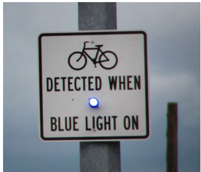
Blue light integrated with a regulatory sign in Portland, OR
