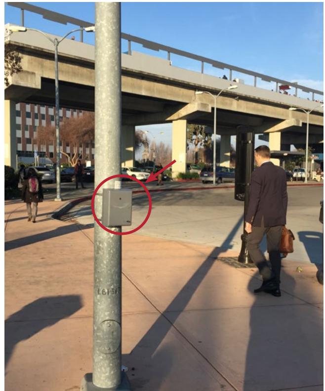
This microwave automated counter counts the volume of pedestrians and bicyclists accessing this rail station in Oakland, CA
