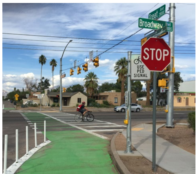
Separate push buttons are typically provided for pedestrians and bicyclists if users have adjacent crossing paths (Tucson, AZ)
