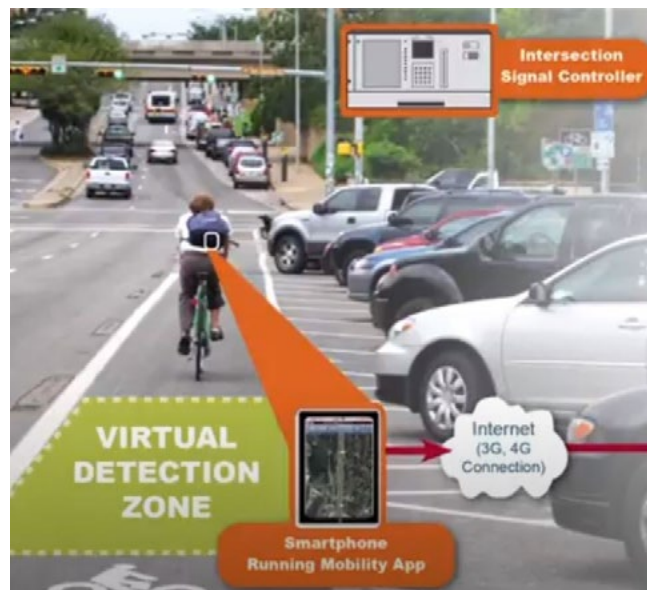
Austin's "Bicycle Mobility App" helps detect bikes at over 70 signalized intersections in the city. This system was deployed in 2015. Source: City of Austin via YouTube
