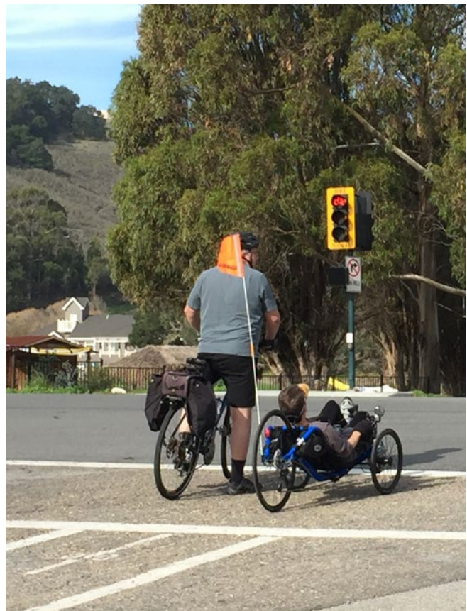
These bicyclists are waiting outside of the loop detector and may not be detected at this signal
