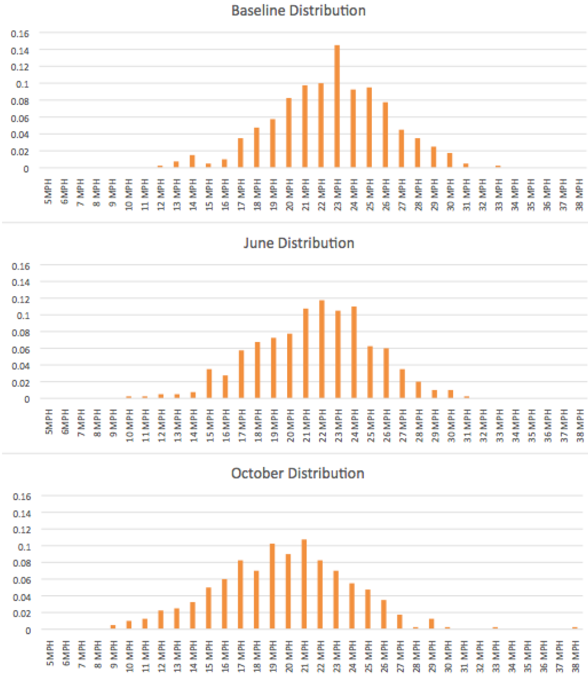
Figure 4.9 The speed distribution at the midblock crosswalk on Main Street in Three Rivers. The top frame shows the distribution of speeds for baseline, the middle frame shows the distribution in June and the bottom frame shows the distribution in October.
