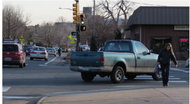
Crashes between pedestrians and right turning vehicles are a common pedestrian crash type in most US and Canadian communities.
