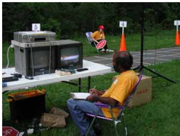
Figure 41. Several video cameras were positioned at strategic points around the braking area.
