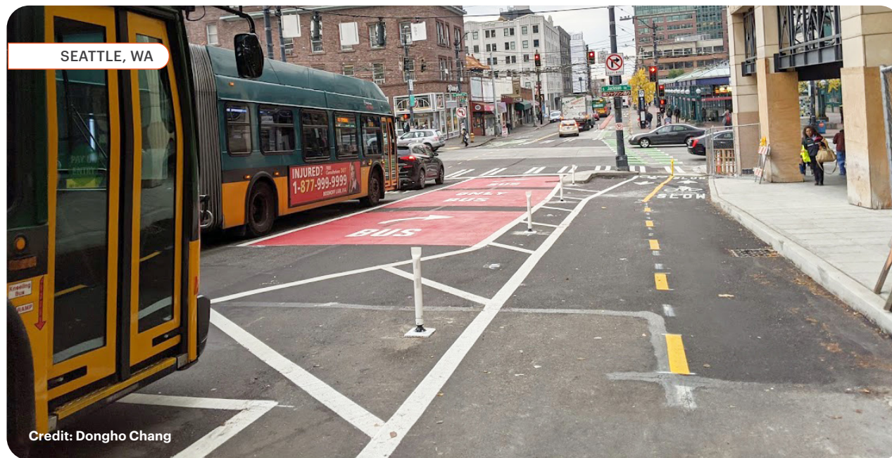
At the bus terminal on King Street in Pioneer Square Seattle there is a bus-only right-turn pocket that ensures buses avoid traffic delays at the start of their route. 74
