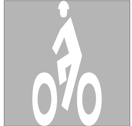
Bicycle pavement marking: helmeted bicyclist symbol
