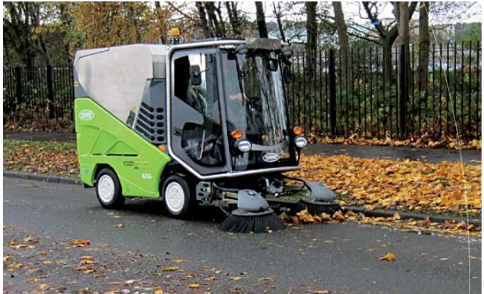
Narrow sweepers like this one can fit into most separated bike lanes (Source: PeopleForBikes)
