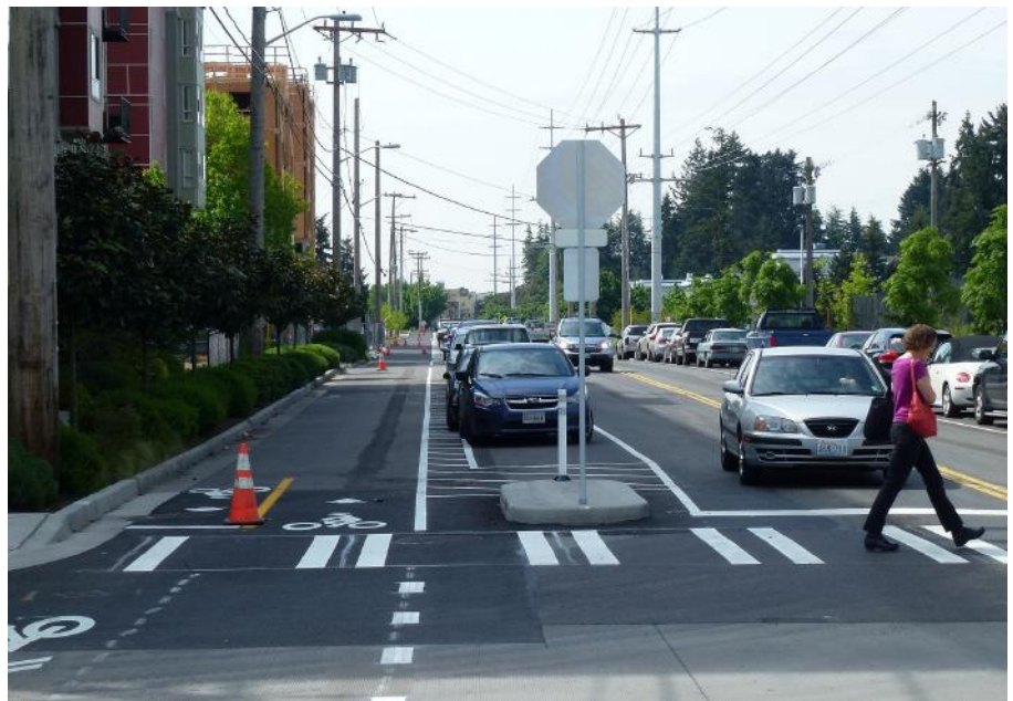
Parked cars provide separation in Seattle, WA. (Source: Seattle DOT)
