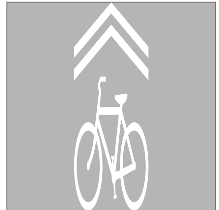
Shared lane marking
