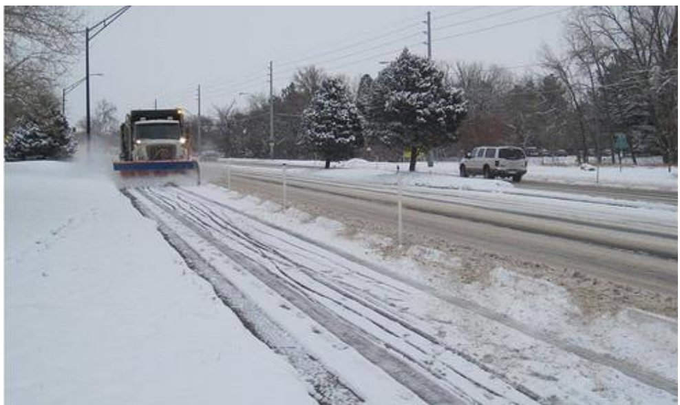
Boulder uses a standard plow that fits in its 2-way Baseline Road separated bike lane. (Source: City of Boulder)
