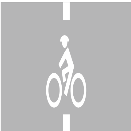
Bike detector pavement marking
