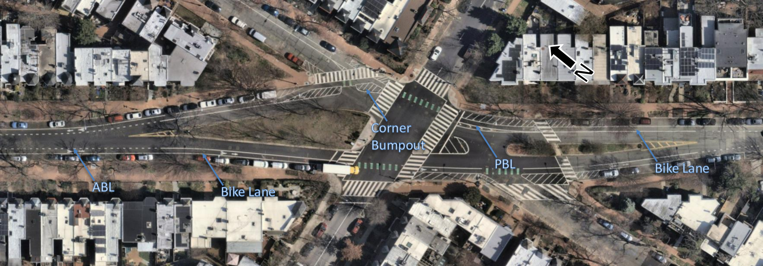
ABLs transition to dedicated bike lanes to protected bike lanes for complex intersection
