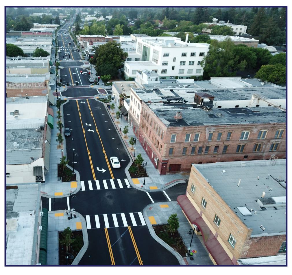
A total of 9 blocks along State Street, the primary arterial roadway in Ukiah, and several connecting side streets were improved. The project also implemented a "road diet" where State Streets' existing four-lanes (two in each direction) were reduced to two-lanes (one in each direction) with center two-way left-turn lanes, parallel parking and wider sidewalks. Construction of the project started in the spring of 2020 and was completed during the COVID-19 pandemic.
