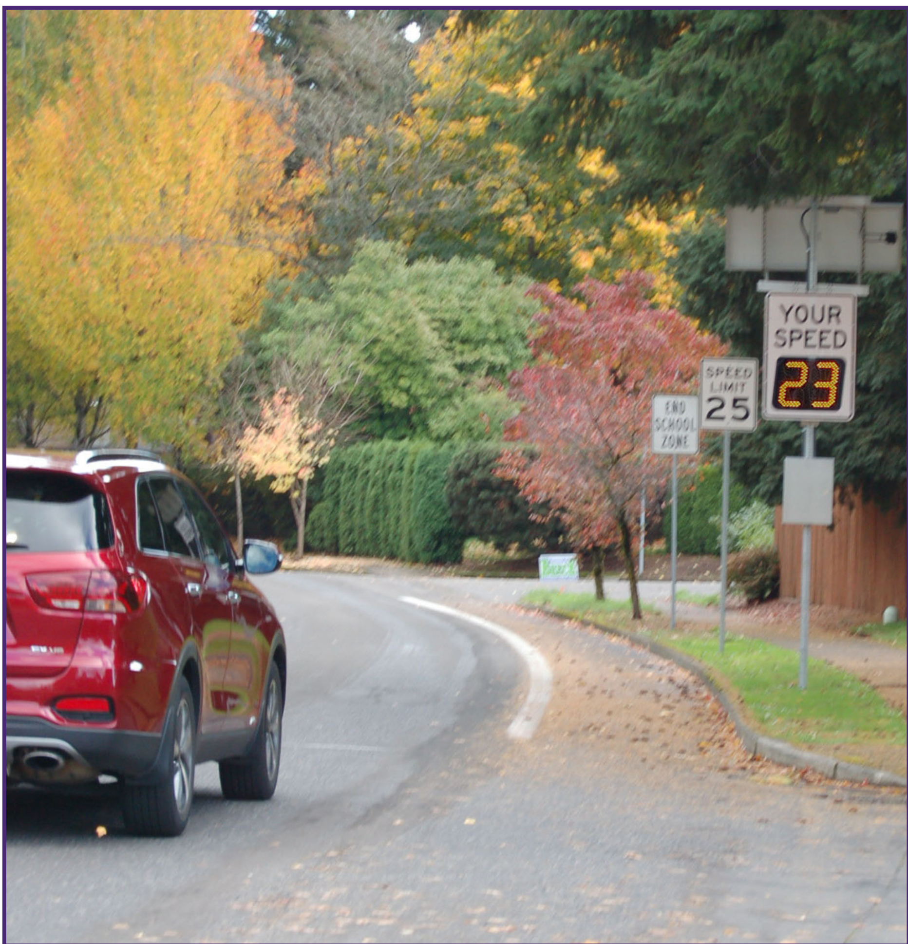
Radar Speed Feedback Signs display actual driver speeds and encourage slower driver speeds. In a 2019 project, they were installed along NE Hearthwood Way to slow drivers approaching controlled intersections.
