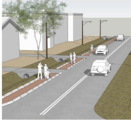
OD-2.1 Rendering of permeable paving sidewalk on one side of the street
