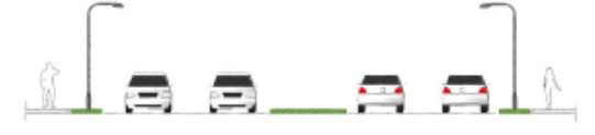
Curb and gutter in a major thoroughfare with buffered sidewalks on both sides
