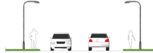
Curb and gutter in a local street with no sidewalks
