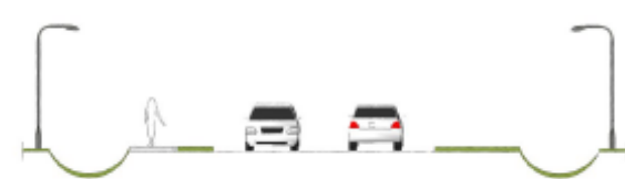
Open ditch next to property line with sidewalk on one side
