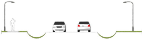
Open ditch next to roadway with sidewalk on one side
