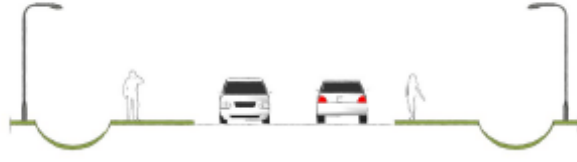
Open ditch next to property line with no sidewalks
