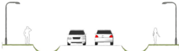
Open ditch between narrow roadway or property line
