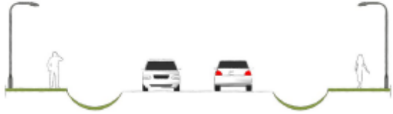
Open ditch next to roadway with no sidewalks
