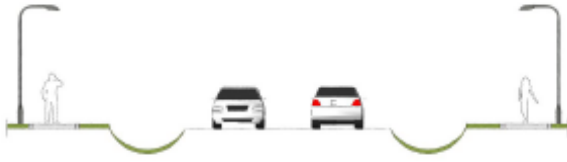
Open ditch next to roadway with sidewalk on both sides
