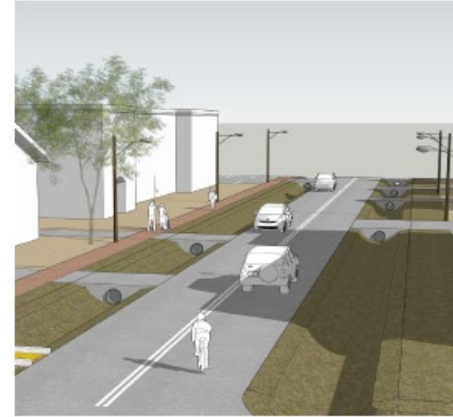
OD-1.1 Rendering of permeable sidewalk on one side of the street next to open ditch
