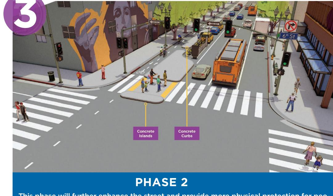
This phase will further enhance the street and provide more physical protection for people walking and bicycling. Proposed upgrades include: concrete islands at intersections; and a concrete barrier along the length of the facility. New curbside management zones are also being considered. Design for this phase is in progress.
