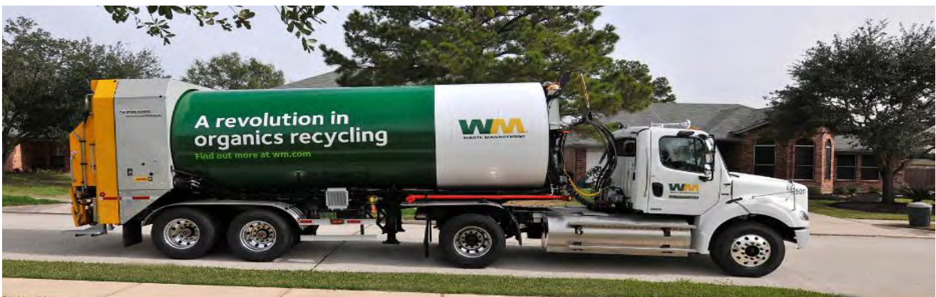
Figure 22: Houston Waste Management deployed German-produced Rotopress refuse trucks with 40 percent larger capacity and 40 percent smaller turn radius than a rigid refuse truck.
