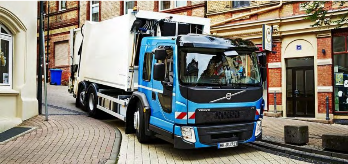
Figure 9: Low-entry cabs and additional “peep” windows in truck cabs let drivers see adjacent people and objects
