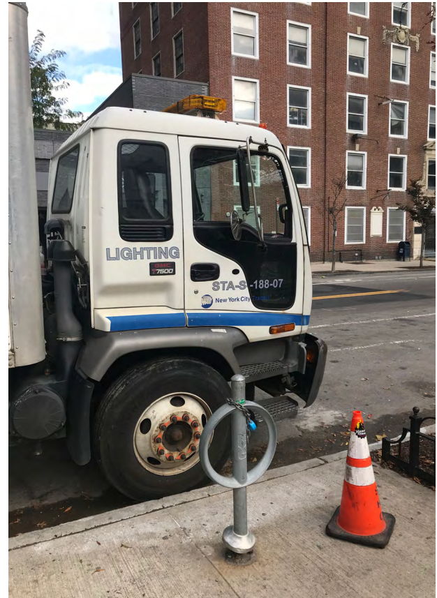
Figure 30: Peeper windows and increased visibility doors can be retrofit into existing vehicles. New York City Metropolitan Transit Agency, New York, NY
