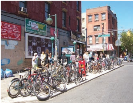
ABOVE: Curb extension with bike parking: North 7th Street, Brooklyn
