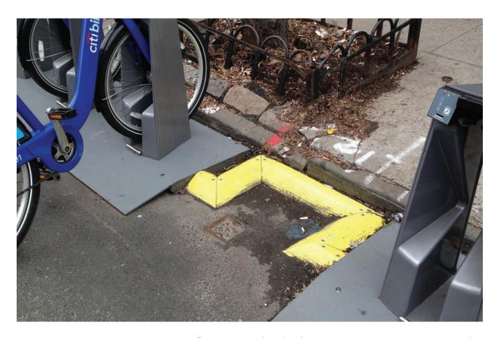
Bridging allows the station to fit around a utility cover and provides additional flexiblity in station design. Citi Bike. New York, NY
