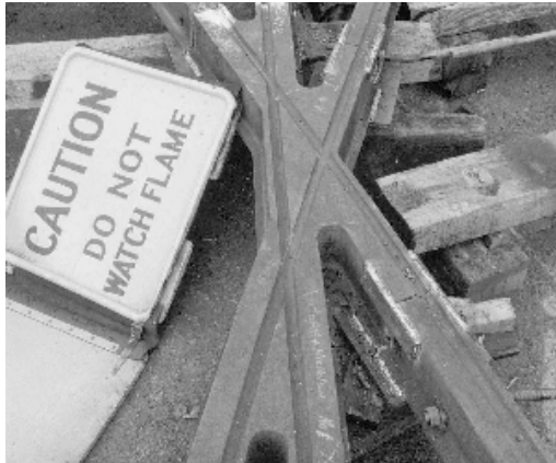
Figure 11. - Cast crossing frog electrically welded to carbon steel grooved rail.
