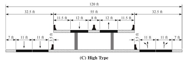
Figure 1-15. Minimum Cross Section and Right of Way for a Two-Lane Flyover. 11
