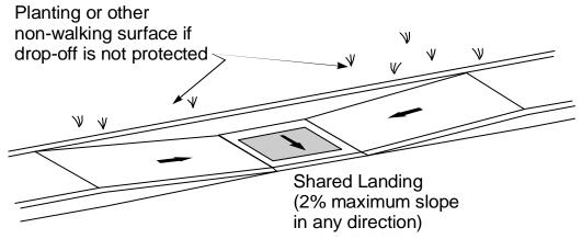
Figure 7-4. Parallel Curb Ramps.
