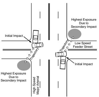
Figure 5-10. Intersection Zones Having Highest Exposure to Secondary Collisions. 11
