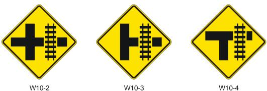
Figure 11-4. Alternative Warning Signs for Use on Roadways Parallel to Railroad Tracks.<sup>9</sup>
