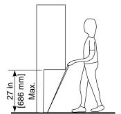
Protruding objects of a height less than or equal to 27 in [686 mm] are detectable and do not require additional treatment.
