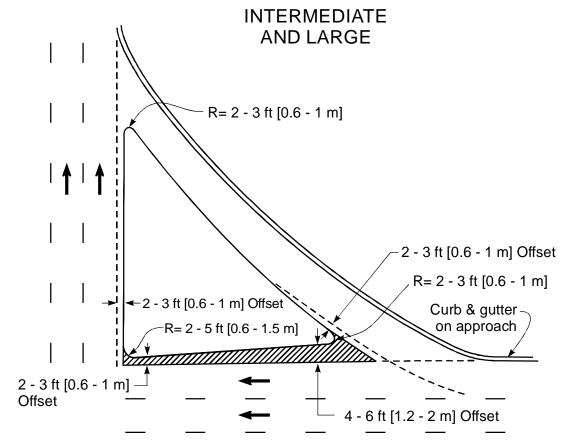
Figure 4-17. Details of Corner Island Designs for Turning Roadways (Urban Locations).
