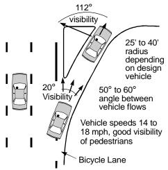
Figure 4-18. Suggested Design for Right-Turn Lane with Island. 11
