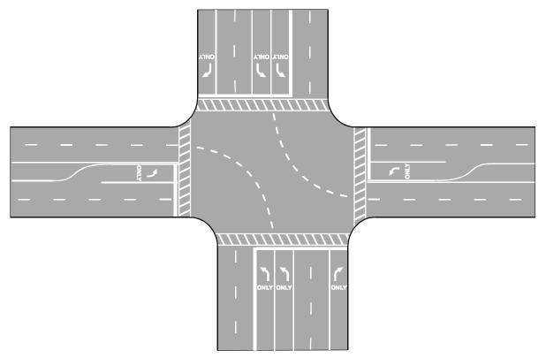
Figure 9-5. Typical Dotted Line Markings to Extend Longitudinal Lane Line Markings.
