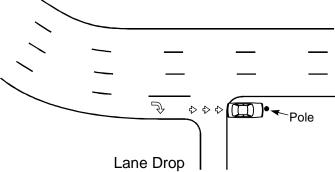
Figure 5-7. Exposure of Vehicle to Utility Pole Downstream of Lane Drop. 11
