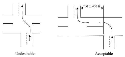
Figure 11-1. Elimination of Jog Crossing Movements by Increasing Separation.
