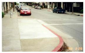
Figure 5-21. Example of a Curb Extension.
