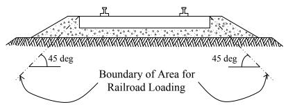
Figure 6-15. Diagram Showing Area Requiring Consideration for Railroad Loading.
