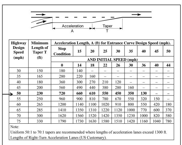
Figure 4-2. Length of Right-Turn Acceleration Lanes (Reproduced from Roadway Design Manual Figure 3-10 < link > ).
