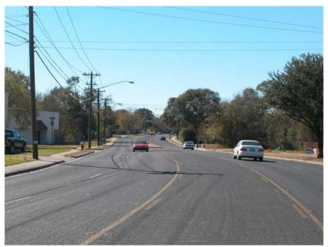
Figure 9-1. Example of Longitudinal Pavement Markings.
