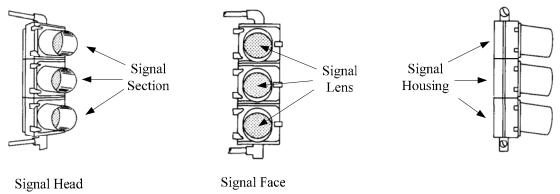
Figure 8-1. Components of a Three-Section Traffic Signal Head.
