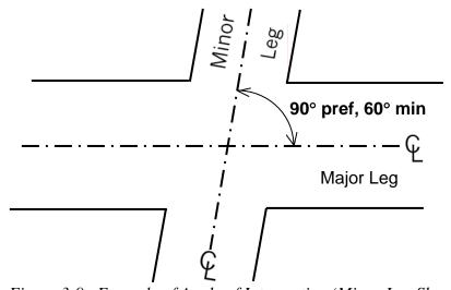
Figure 3-9. Example of Angle of Intersection (Minor Leg Skewed to the Right).
