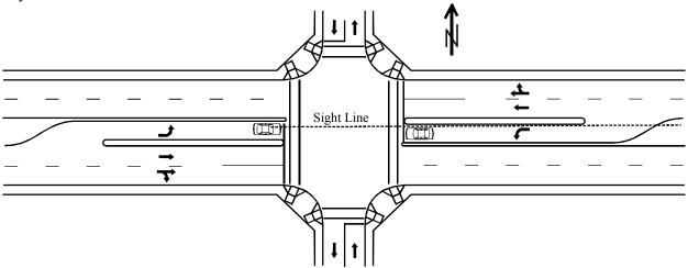
Figure 4-14. Proposed Design for Offset Left-Turn Lane.
