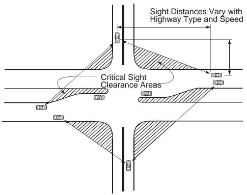
Figure 5-15. Plant Use in Intersection Areas Must Be Limited to Low-Growing Varieties to Provide for a Clear Sight Triangle. <sup>12</sup>
