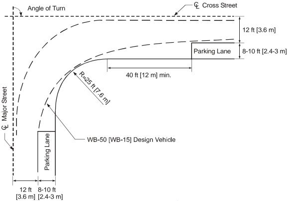
Figure 3-8. Effective Radius with Parking Restriction.<sup>4</sup>
