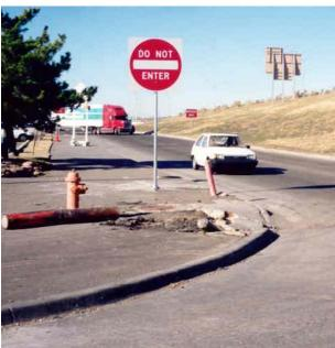
(A) Stop Sign and Back of Do Not Enter Sign (B) Do Not Enter Sign Figure 10-14. An Example of a Do Not Enter Sign Obscuring the Shape of a Stop Sign.
