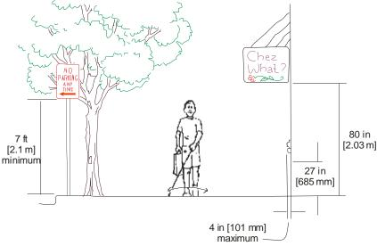
Figure 10-1. Sidewalk Free of Protruding Objects.<sup>5</sup>
