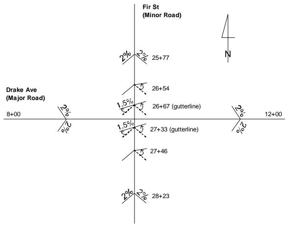
Figure 6-4. Fir Street Cross Section Transition.
