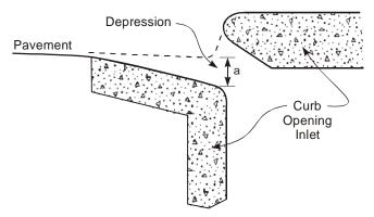
Figure 6-9. Depression at Curb Opening Inlet.
