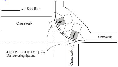
Figure 7-2. Perpendicular Curb Ramp.
