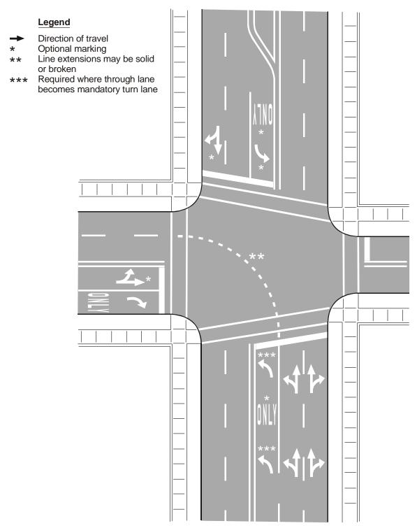
Figure 9-10. Typical Lane Use Control Word and Symbol Markings.
