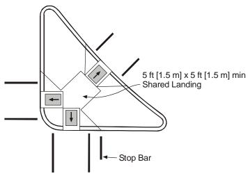
Figure 4-24. Typical Layout of Curb Ramps at a Channelizing Island. 15
