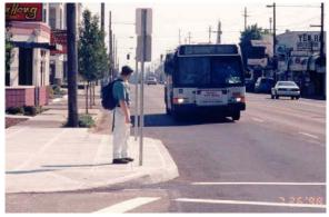
Figure 5-23. Example of Bus Bulb.
