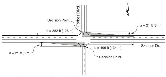
Figure 3-8. Case B2 – Sight Triangles for Right-Turning Passenger Cars.
