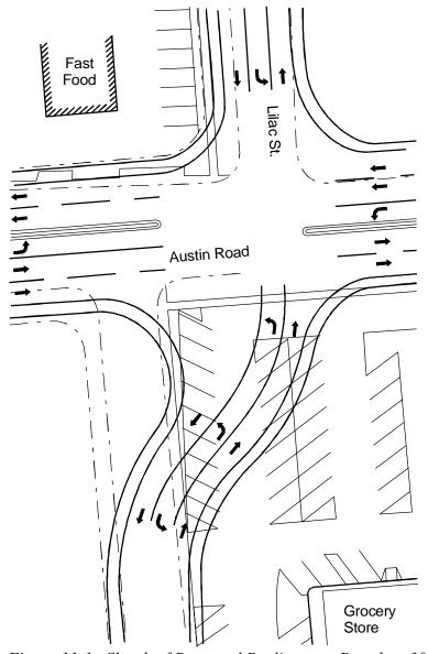
Figure 11-1. Sketch of Proposed Realignment Based on 30 mph [48 km/h] Design Speed.
