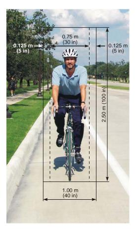
Figure 2-3. Bicyclist Operating Space (Based on Data in the AASHTO Guide for the Development of Bicycle Facilities<sup>9</sup>).
