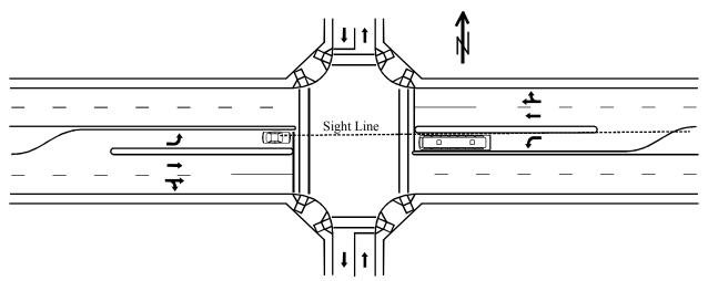
Figure 4-15. Proposed Design for Offset Left-Turn Lane with Bus.
