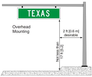
Figure 10-4. Overhead Street Name Sign on Mast Arm Post.
