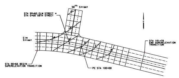
Figure 3-34. Contour of Intersection.
