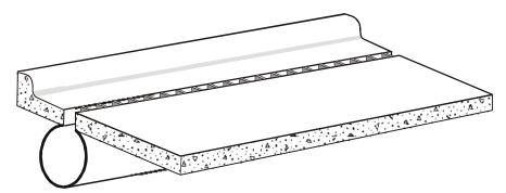
Figure 6-14. Slotted Drain.
