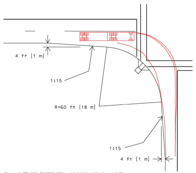
Figure 3-37. WB-50 [WB-15] on 60-ft [18 m] Radius with Taper.
