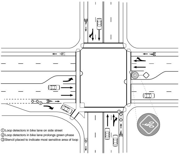
Figure 8-14. Signalized Intersection Sensitive to Bicycles (Based on Oregon Bicycle and Pedestrian Plan). 19
