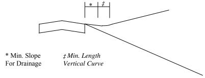
Figure 6-4. Normal Crown on Major Roadway, Stop Condition on Minor Roadway.<sup>6</sup>
