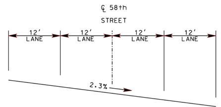
Figure 3-33. Cross Section of 58<sup>th</sup> Street Entering Intersection (STA 0+31).
