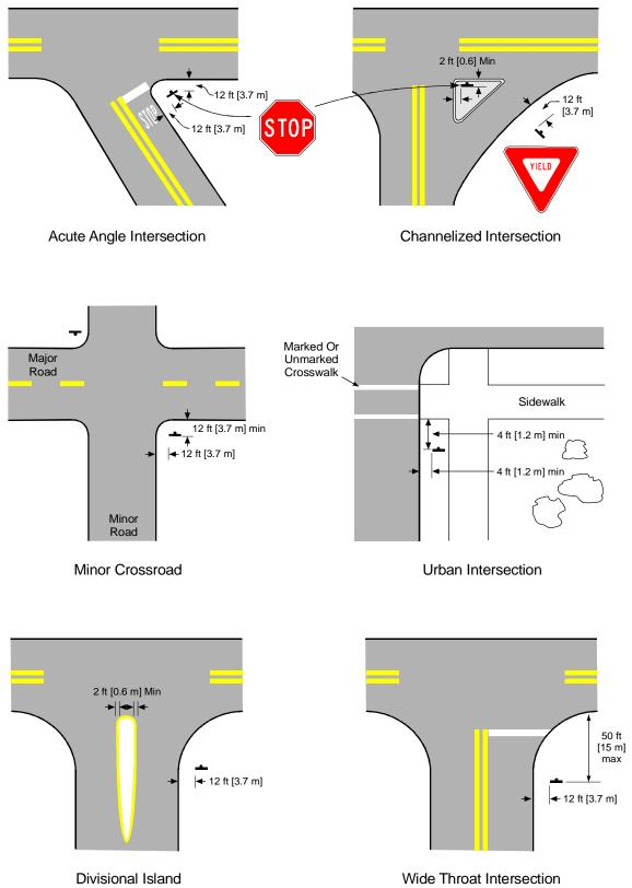
Figure 10-10. Typical Locations for Stop Signs at Intersections. <sup>1</sup>
