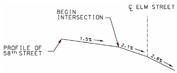
Figure 3-31. Revised Profile of 58<sup>th</sup> Street as It Meets Elm Street's Cross Slope.
