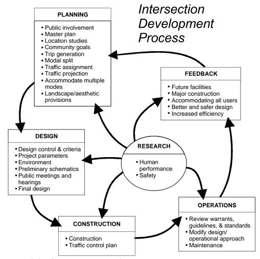
Figure 1-1. The Intersection Development Process.
