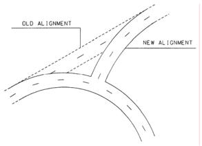
Figure 3-4. Realignment of Tangent Roadway at Intersection.<sup>3</sup>
