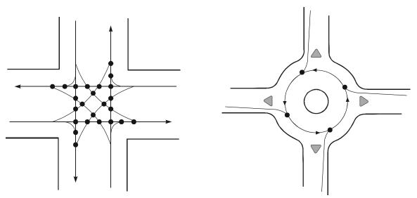
Figure 1-4. Comparison of Conflict Points at a Traditional Four-Leg Intersection and a Roundabout.<sup>3</sup>
