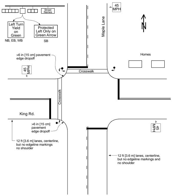
Figure 2-1. Condition Diagram.
