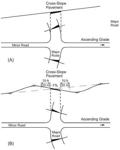
Figure 3-12. Coordination of Vertical Alignments on Horizontal Curves. 10
