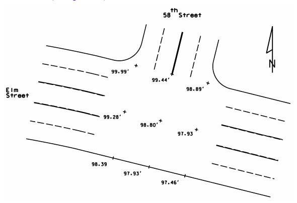
Figure 3-32. Elevations in Intersection.
