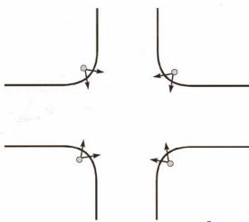
Figure 8-4. Post-Mounted Signals.<sup>7</sup>
