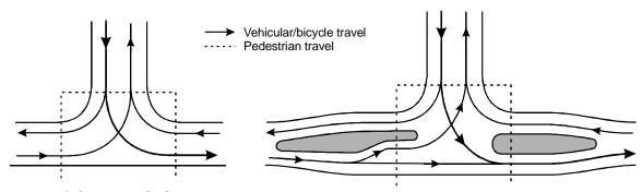
Figure 1-3. Typical Three-Leg Intersection.
