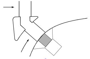
Figure 4-12. Reduction of Pedestrian Exposure with Raised Islands.<sup>8</sup>
