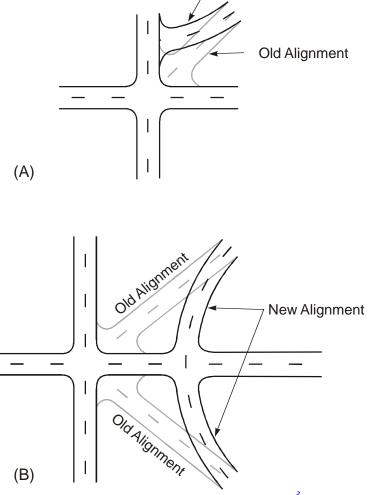
Figure 3-5. Realigning Multileg Intersections.<sup>3</sup>
