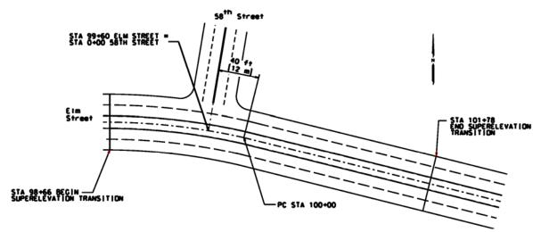
Figure 3-30. Revised Layout of Superelevation Transition.
