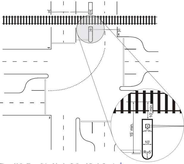
Figure 11-8. Channelizing Island at Railroad Grade Crossing.<sup>8</sup>
