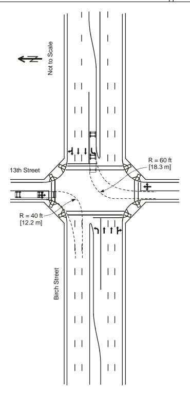
Figure 4-4. Design Overlaid with WB-50 [WB-15] Truck Template.
