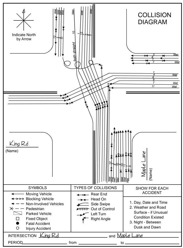
Figure 2-2. Collision Diagram.
