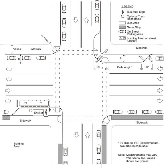
Figure 5-24. Typical Bus Bulb Dimensions. 15
