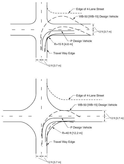
Figure 3-6. Effect of Curb Return Radius on Right Turning Paths (R=15 ft [4.6 m] and R=40 ft [12.2 m]).
