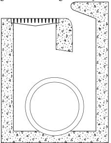
Figure 6-13. Example of Combination Inlet.
