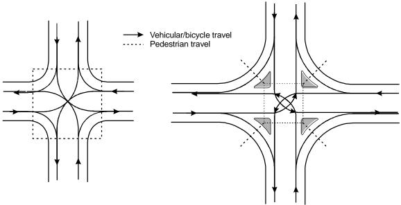
Figure 1-5. Typical Four-Leg Intersections.
