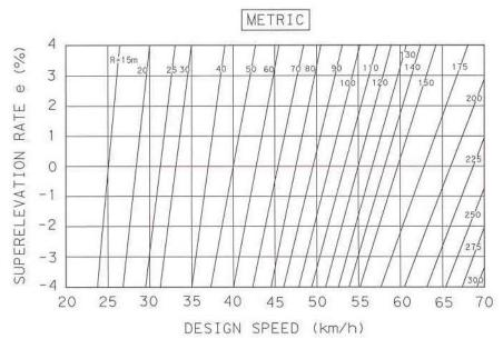
Figure 3-27. Relationship of Radius, Superelevation Rate, and Design Speed for Low-Speed Urban Street Design (Reproduction of Roadway Design Manual Figure 2-2 < link>).
