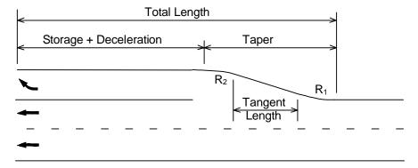
$R_1 = 2R_2$  (Approximate) Tangent Length = (1/3 to 1/2)(Taper Length)
