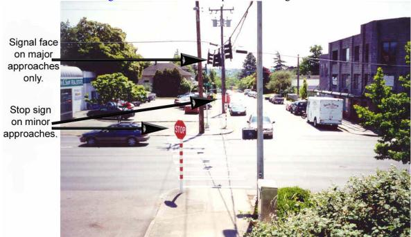
Figure 7-37. Example of a Half Signal in Seattle, Washington.
