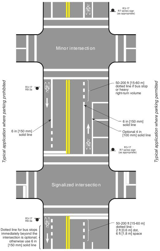
Figure 4-27. Bicycle Lane Marking Examples.<sup>9</sup>
