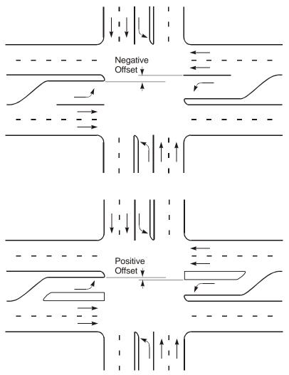
Figure 4-4. Negative and Positive Offsets of Left-Turn Lanes.<sup>4</sup>
