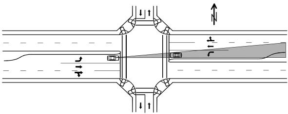
Figure 4-13. Existing Intersection Showing Visual Blocking.
