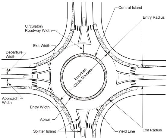
Figure 1-3. Example of Roundabout.
