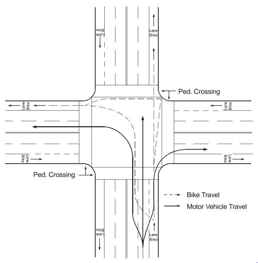
Figure 4-29. Typical Bicycle and Motor Vehicle Paths at Major Intersections.<sup>9</sup>
