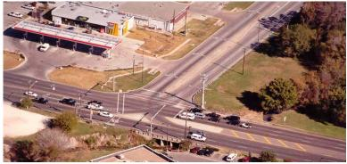
Figure 1-4. Aerial Photograph of a Channelized T-Intersection.
