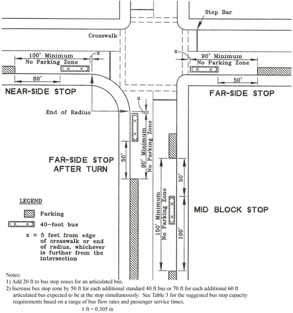
Figure 5-25. Typical Types of and Dimensions for On-Street Bus Stops. 16
