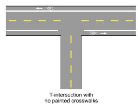
Figure 4-28. Example of Bicycle Lane Marking at T-Intersections.<sup>9</sup>
