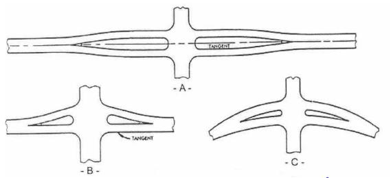
Figure 4-19. Layouts for Addition of Divisional Islands at Intersections.<sup>2</sup>
