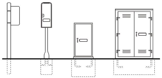
Figure 8-11. Types of Controller Cabinet Mountings.<sup>7</sup>
