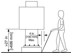
When an obstruction of a height greater than 27 in [686 mm] from the surface would create a protrusion of more than 4 in [100 mm] into the pedestrian circulation area, construct additional curb or foundation at the bottom to provide a maximum 4 in [100 mm] overhang.
