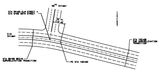
Figure 3-28. Layout Showing Superelevation Transition Placement.
