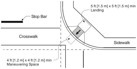
Figure 7-7. Diagonal Curb Ramp.
