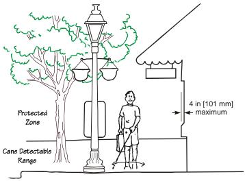
Figure 5-6. Post-Mounted Objects (Post-Mounted Objects Seen in Elevation, Dimensioned to Indicate 4 inch [101 mm] Maximum Protrusion). 10
