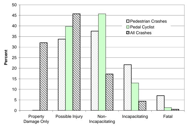
Figure 2-5. Pedestrian and Bicyclist Accident Severity (Texas Urban On- and Off-System Roadways 1998–2000).
