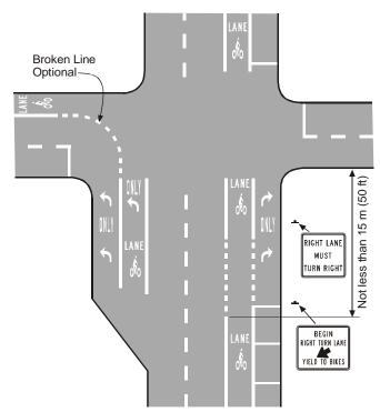
Figure 9-13. Typical Intersection Pavement Markings with Designated Bicycle Lane with Left-Turn Area, Heavy Turn Volumes, Parking, One-Way Traffic, or Divided Highway.
