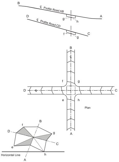
Figure 6-7. Cross Section Held Constant on Both Roadways, Technique Not Recommended Because It Results in an Uncomfortable Ride on Both Roadways.<sup>7</sup>
