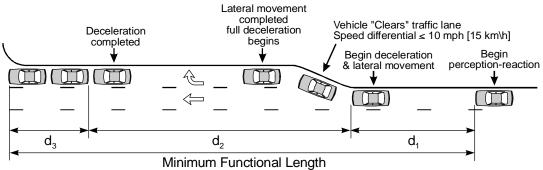
Figure 1-8. Elements of the Functional Area of an Intersection. 18
