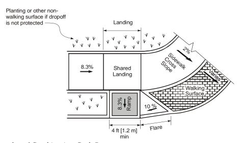
Figure 7-6. Examples of Combination Curb Ramps.
