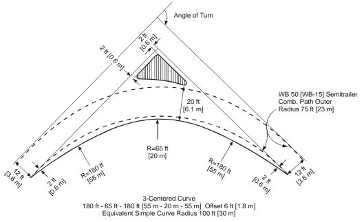
Figure 4-9. Minimum Turning Roadway Design to Accommodate WB-50 [WB-15] with Corner Island at Urban Locations.<sup>2</sup>
