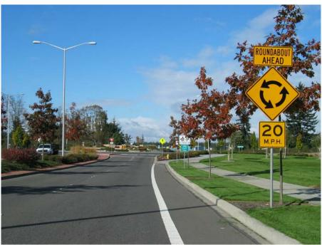
Figure 1-6. Roundabout Advance Warning Sign Example.
