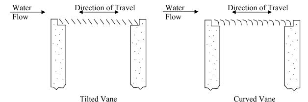
Figure 6-12. Tilted Vane (or "Bar") and Curved Vane Grate Inlets.
