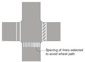
Figure 9-7. Crosswalk Marking Options.<sup>1</sup>
