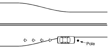
Figure 5-8. Placement of Pole Downstream of Roadway Narrowing. 11
