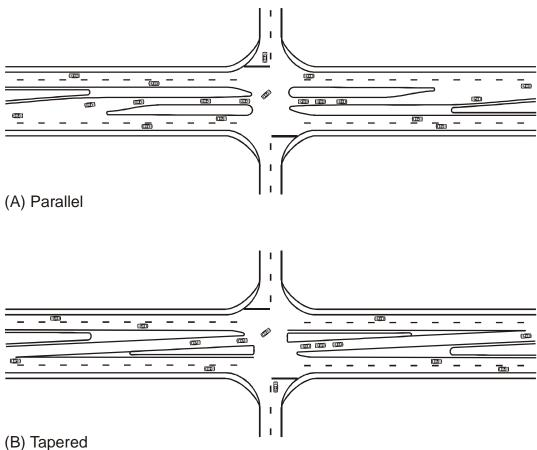
Figure 4-6. Parallel and Tapered Offset Left-Turn Lane.<sup>2</sup>
