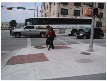
Figure 7-3. Photo of Perpendicular Curb Ramps.
