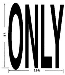
Figure 9-12. Typical Elongated Letters for Word Pavement Markings.
