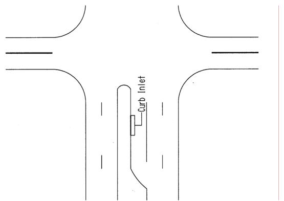
Figure 6-8. Median with Inlet Placed to Avoid Trapping Water.
