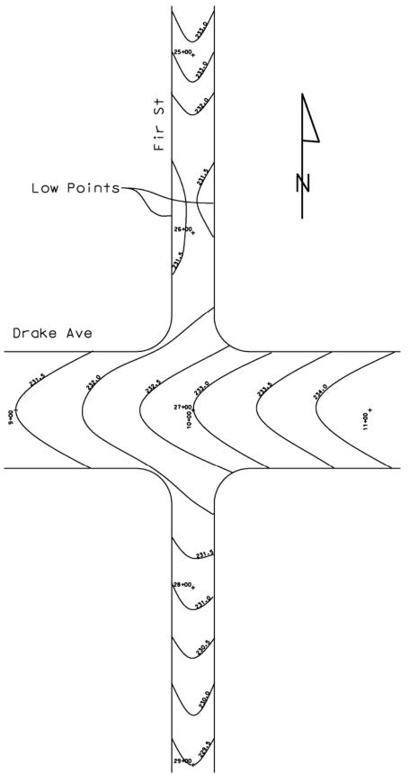
Figure 6-5. Contour Plot of Intersection.
