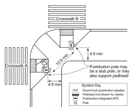
Figure 8-13. Recommended Placement for Pedestrian Push Buttons — Integrated APS in New Construction. 14
