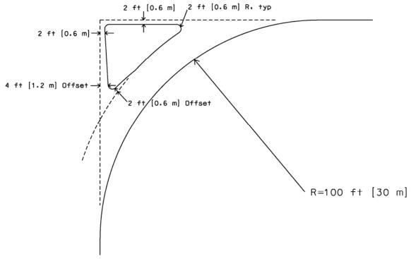
Figure 4-22. 100-ft [30 m] Turning Radius and Island.
