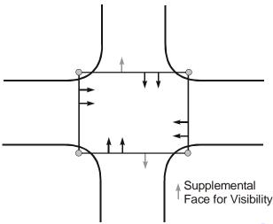
Figure 8-7. Span Wire Mounting: Box Span.<sup>7</sup>
