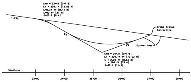
Figure 6-2. Vertical Profile of North Section of Fir Street.
