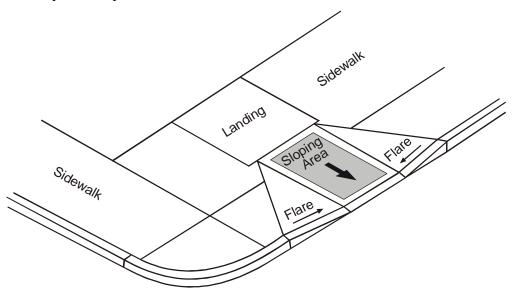
Figure 7-1. Components of a Curb Ramp.
