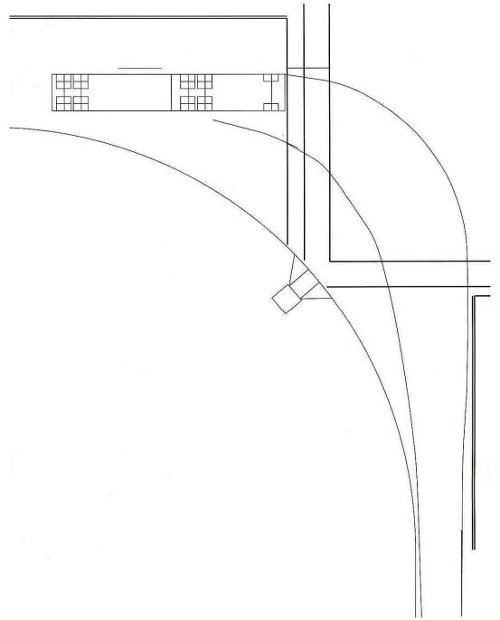
Figure 3-35. WB-50 [WB-15] Truck on 100-ft [30 m] Radius Curve.
