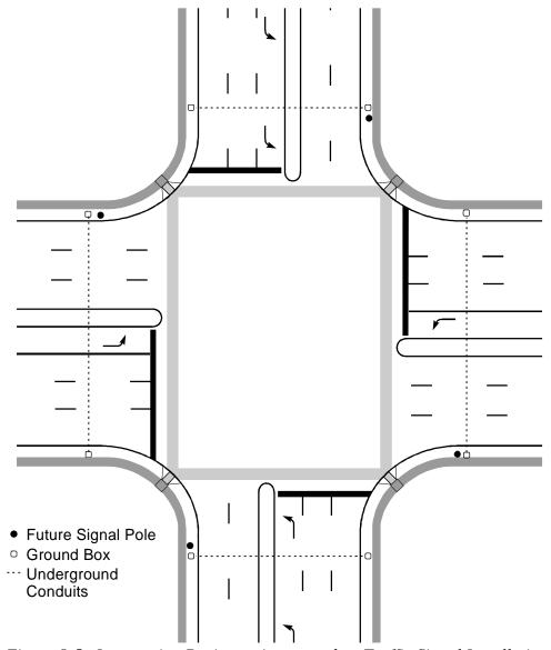
Figure 8-5. Intersection Design to Accommodate Traffic Signal Installation.
