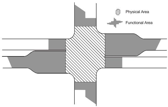
Figure 1-7. Functional Area of an Intersection. <sup>18</sup>
