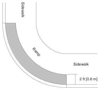
Figure 7-8. Example of a Blended Transition.
