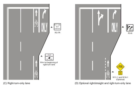
Figure 4-30. Illustration of Bicycle Lane Treatments at Location with Right-Turn Lane.
