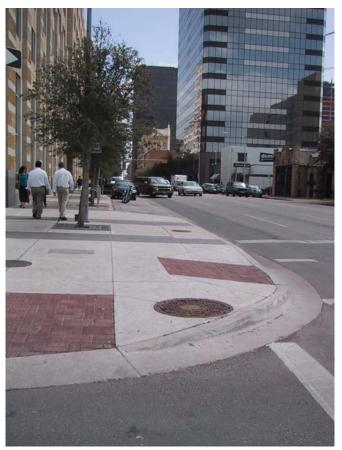
Figure 5-31. Example of Manhole Outside Pedestrian Access Route.
