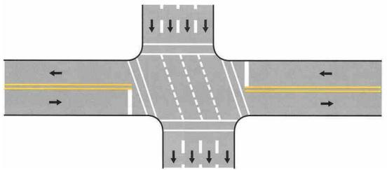
Figure 9-4. Typical Pavement Marking with Offset Lane Lines Continued through the Intersection. <sup>1</sup>
