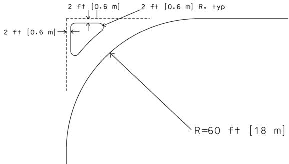
Figure 4-24. 60-ft [18 m] Turning Radius and Island.
