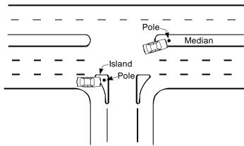
Figure 5-9. Inappropriate Location of Poles within a Traffic Island or Median. 11
