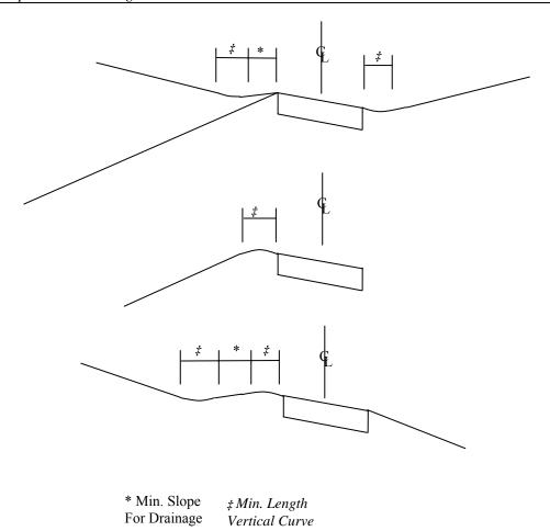
Figure 6-5. Superelevated Major Roadway, Stop Condition on Minor Roadway.<sup>6</sup>
