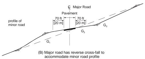
Figure 3-11. Coordination of Vertical Alignments on Horizontal Tangent. 10
