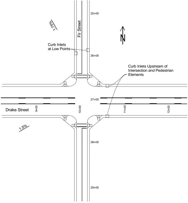
Figure 6-6. Final Intersection Layout.
