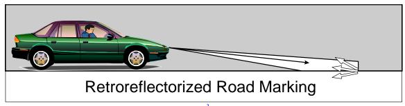
Figure 9-3. Light Reflection Characteristics.<sup>3</sup>
