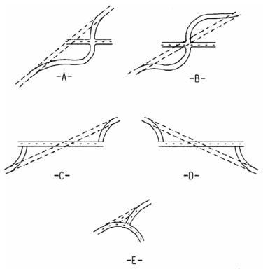
Figure 3-10. Realignment Options at Intersections.<sup>3</sup>
