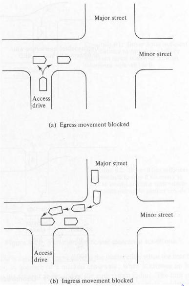
Figure 11-10. Driveways Blocked by Intersection Queue.<sup>2</sup>
