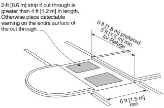
Figure 4-26. Cut through at Raised Median. 15
