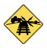
Figure 11-3. Low Ground Clearance Highway-Rail Grade Crossing Sign (W10-5).9
