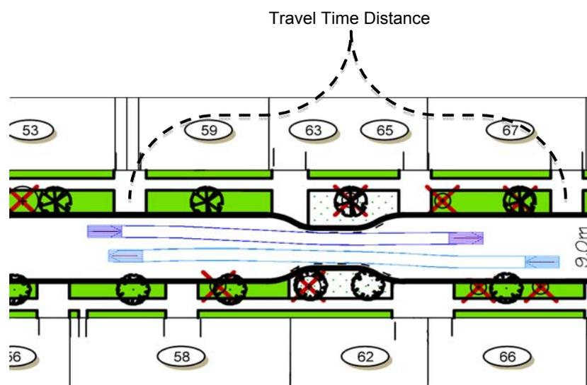
Figure 5: Two-way vehicle movements at the pinch-point
