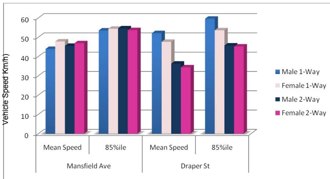
Figure 7: Travelling Speeds of Male and Female Drivers at Pinch-points
