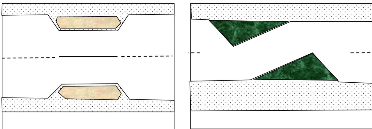
Figure 1: Typical 2-way Pinch-Point and 1-way Chicane
