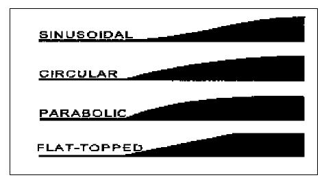
Figure 3. Commonly Used Speed Hump Profiles (Ewing, 1999)
