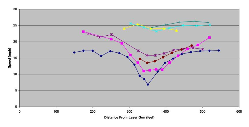
Figure D3. Roosevelt Drive Northbound Temporary 30 mph Speed Table Speed Profiles.
