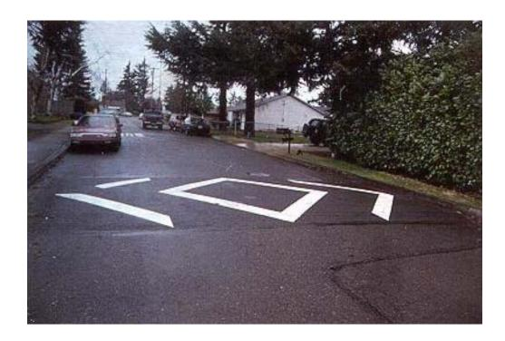
Figure 1. Typical Speed Hump (Traffic Calming for Communities, 2001)
