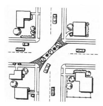
Figure A3: Diagonal Diverter (4).
