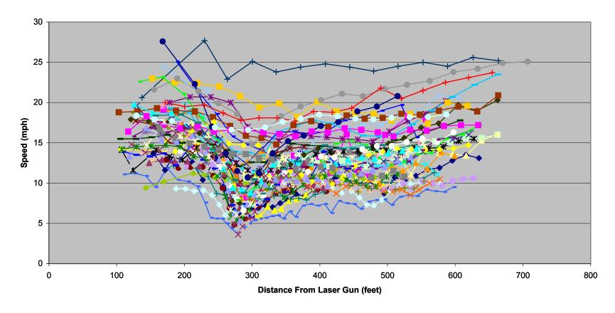
Figure D14: Canal Shore Drive Temporary 25 mph Speed Hump Speed Profiles
