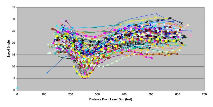
Figure D11: Redwood Drive Temporary 30 mph Speed Table Speed Profiles
