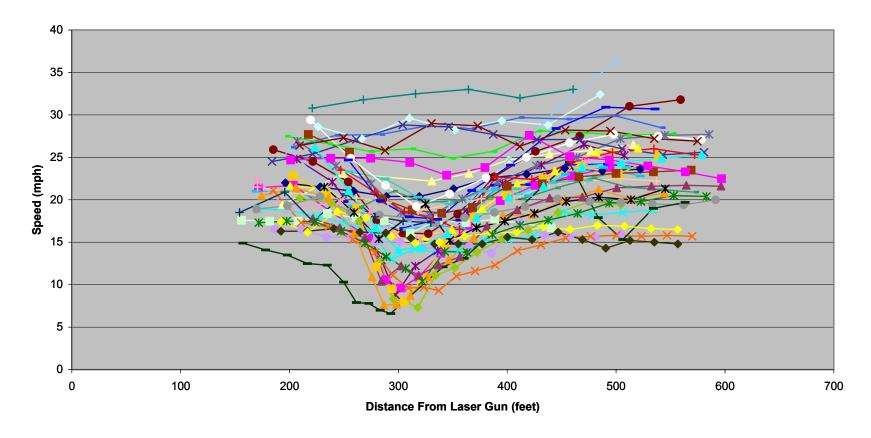
Figure D6: Roosevelt Drive Southbound Temporary 25 mph Speed Hump Speed Profiles
