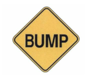
Figure 5. Typical W8-1 BUMP Warning Sign (FHWA, 1988)
