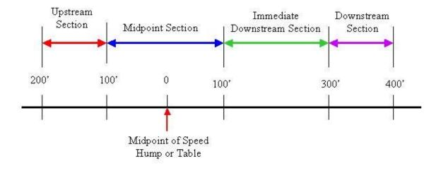
Figure 30. Schematic of Section Locations
