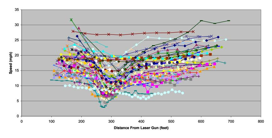
Figure D15: Canal Shore Drive Temporary 30 mph Speed Table Speed Profiles
