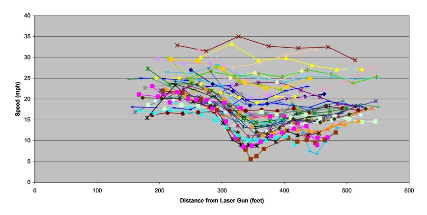
Figure D2. Roosevelt Drive Northbound Temporary 25 mph Speed Hump Speed Profiles.
