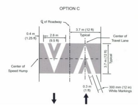
Figure 9. Typical Speed Hump Pavement Markings Shown in the MUTCD (FHWA, 1988)
