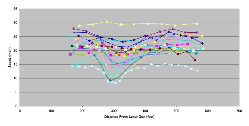
Figure D7: Roosevelt Drive Southbound Temporary 30 mph Speed Table Speed Profiles
