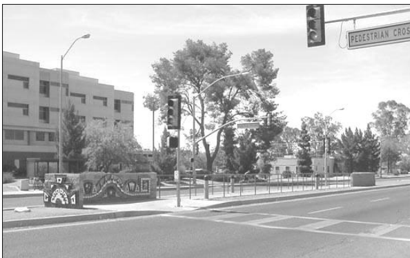
A PELICAN signal, or PE destrian L ight C ontrol A ctivated, uses a standard traffic signal; the signal is always green when not in use and uses a standard yellow to red progression when activated. Usually used for highest volume crossings.
