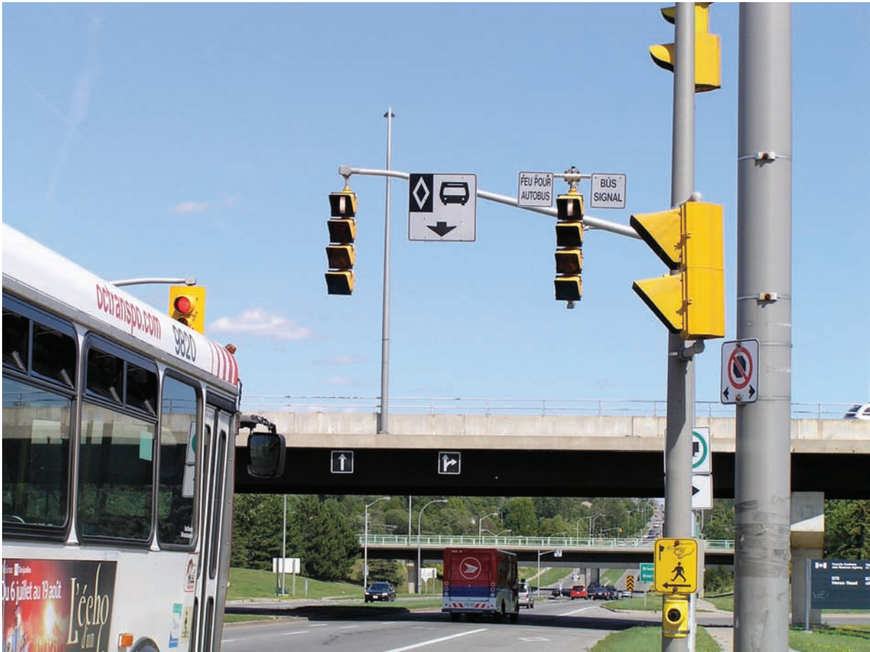
Figure 43 Transit “Cigar” Signal (Top Signal Head)
