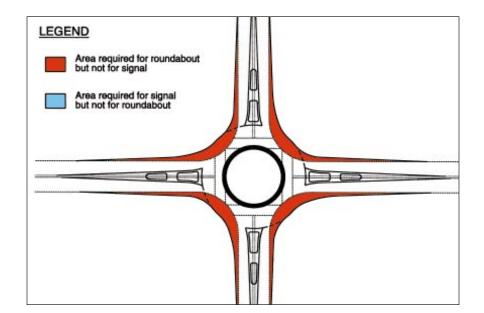
**Exhibit 3-15.** Area comparison: Urban compact roundabout vs. comparable signalized intersection.
