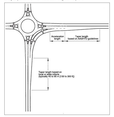
**Exhibit 6-42.** Configuration of right-turn bypass lane with acceleration lane.
