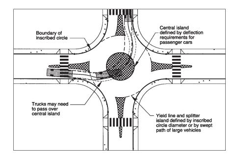
Mini-roundabouts should only be considered in areas where all approaching road-ways have an 85th-percentile speed of less than 50 km/h (30 mph). In addition, mini-roundabouts are not recommended in locations in which high U-turn traffic is expected, such as at the ends of street segments with access restrictions. Miniroundabouts are not well suited for high volumes of trucks, as trucks will occupy most of the intersection when turning.
