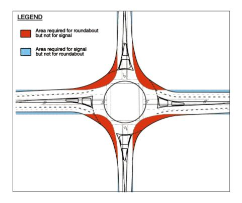
**Exhibit 3-18.** Area comparison: Urban flared roundabout vs. comparable signalized intersection.
