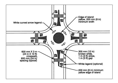
**Exhibit 7-21.** Sample pavement marking plan for a mini-roundabout.
