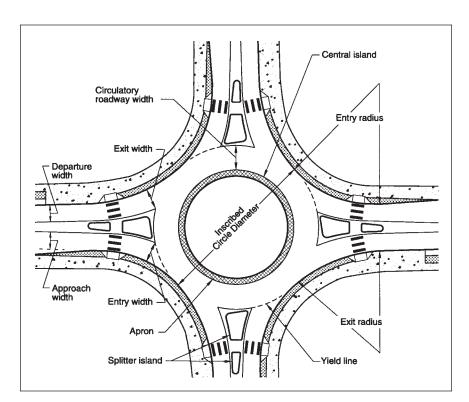
**Exhibit 6-1.** Basic geometric elements of a roundabout.
