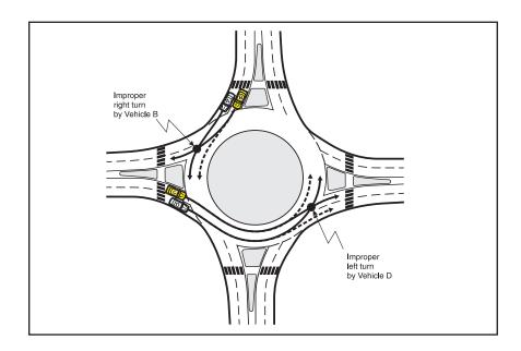
As with single-lane roundabouts, the most severe vehicular crossing conflicts are eliminated and replaced by less severe merging conflicts. The additional conflicts unique to multilane roundabouts are generally low-speed sideswipe conflicts that typically have low severity. Therefore, although the number of conflict points increases at multilane roundabouts when compared to a single lane roundabouts, the overall severity of conflicts is generally less than alternative intersection control.
