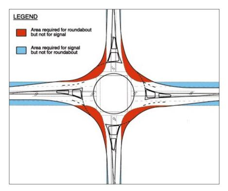
ing roundabouts against other forms of intersections and traffic control, such as comparing a roundabout with a signalized intersection.
