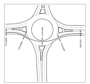
**Exhibit 6-6.** Fastest vehicle path through double-lane roundabout.
