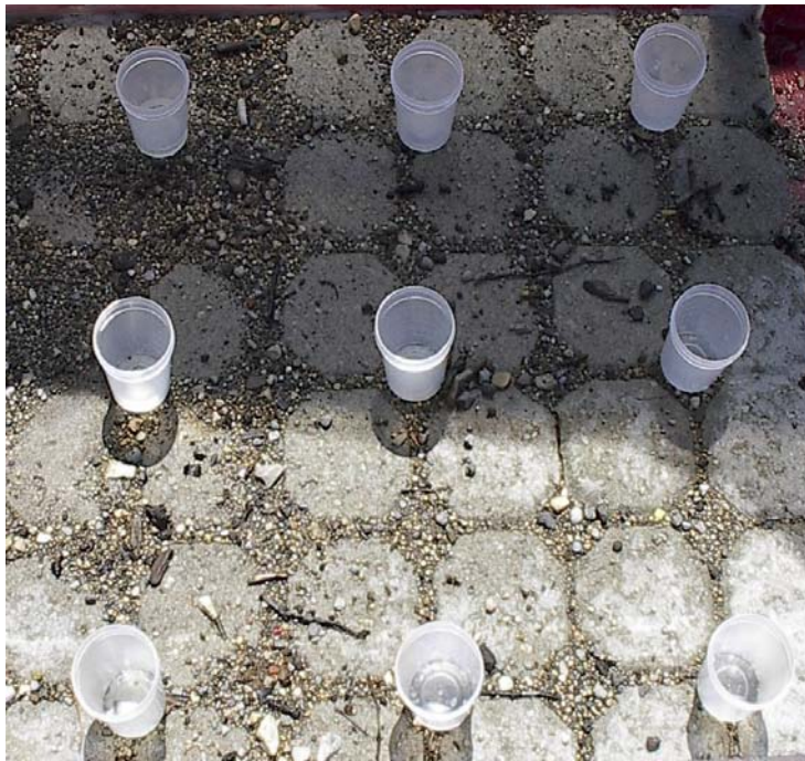
Figure 4. Permeable pavement surface with applied street dust and dirt (The containers are used for rain sampling).
