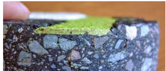
(top) Ease of installation is a significant benefit of the heat applied inlay in lieu of pavers.
