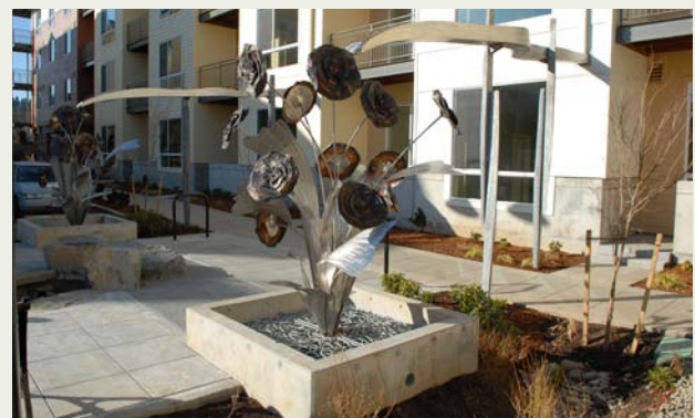
North Main Village, Milwaukee. Stormwater is the featured design element for this residential courtyard. Water from rooftops is conveyed by steel scuppers into decorative planters to meandering runnels and water quality swales.
