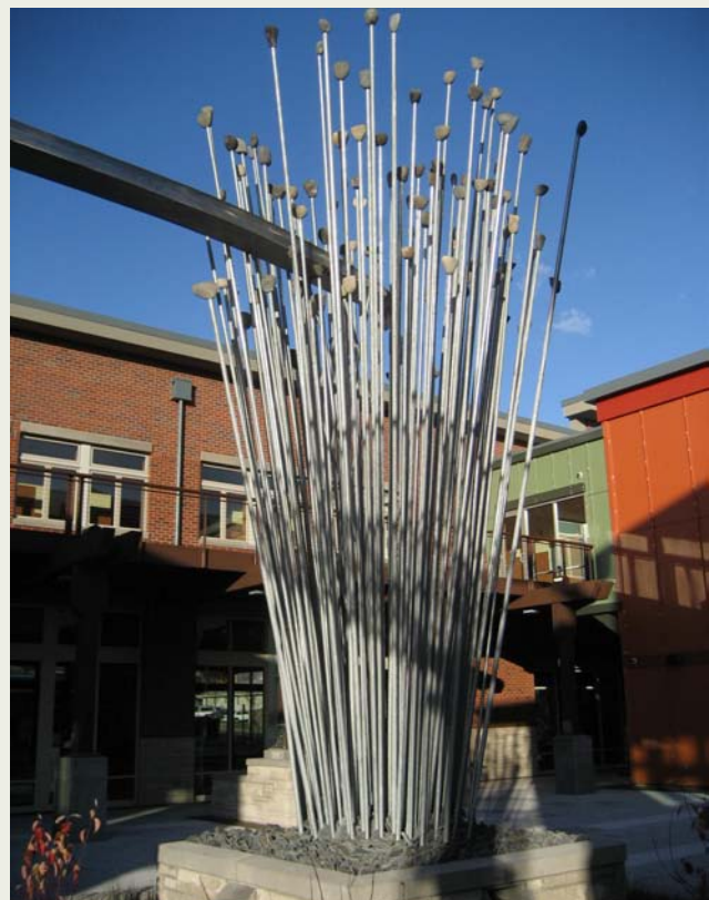
Block 11, Washougal, WA. Stormwater from surrounding rooftops is directed into the plaza's vertical sculpture before entering flow-through planters.
