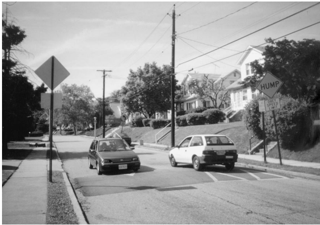
FIGURE 1 Two vehicles slow down as they pass over speed hump.
