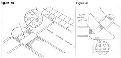
Cut-through medians should be at least 1.525 m (60 in) wide and should include 610 mm (24 in) strips of detectable warnings at both ends.
