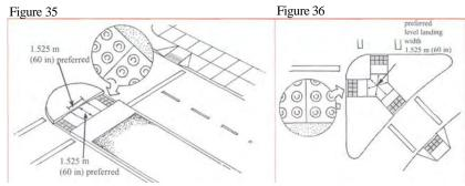
A ramped median should have a level landing that is 1.5 m (5 ft) level landing.
