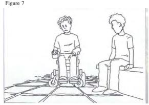
The space between the jointed surface causes wheelchair casters to swivel and catch and greatly increases the rolling resistance.
