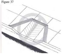
Potential Problem: Grooves are not the equivalent of a detectable warning because they are not detectable underfoot.
