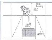
The 1.2 m (4 ft) width of this curb ramp provides sufficient turning space for this wheelchair user. The maximum slope of the flares at this curb ramp should be 10 percent. Measured at the face of the curb.
