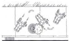
In areas of steep terrain, a wide sidewalk allows wheelchair users to travel in a zigzag motion which reduces the grade they must travel, although the overall distance of their trip is increased.
