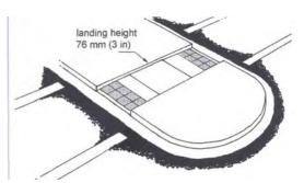
GOOD DESIGN: The height of this median does not exceed 76 mm (3 in). This design allows for the construction of shorter curb ramps and a longer level landing.
