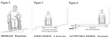
users traveling on a sidewalk with a cross slope greater than 2% use more energy to to offset the force of gravity that directs them towards the curb and into the street
