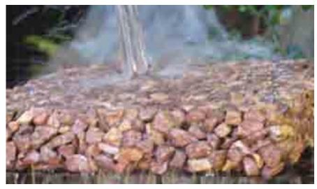
Voids in between stones allow water to pass through (note: for demonstration purposes, this example shows a clear resin, not asphalt, to bind the aggregate particles)
