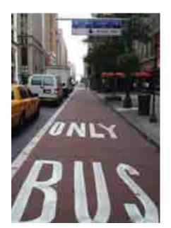
Red, curb—aligned, on—street busway with "soft separation" from traffic: 34th Street, Manhattan
