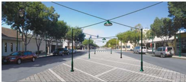
Redesign of travel lanes, introduction of center-of-street diagonal parking, and pedestrian-scale lighting (visualization)
