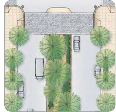
Functional and aesthetic improvements result from the manual's guidance for new geometries, better planting, improved streetscape layout, and stormwater infrastructure such as rain gardens and permeable paving.
