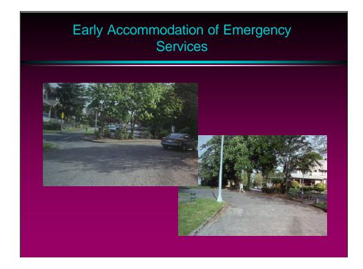
Truncated diverter in upper left and traversable diverter in lower right (with fire hydrants on both sides)
