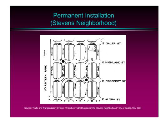
Permanent installation -- diverters replaced by circles at one end of each street Seattle's first application of traffic circles and half closures, now the mainstays of its program
