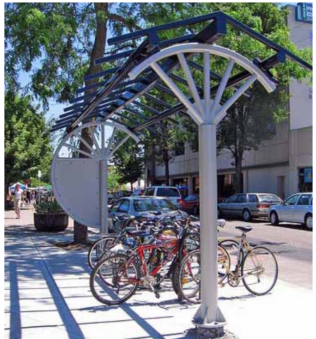
Portland has also built curb extensions putting the parking at sidewalk level. This design, with covered bicycle parking, is called a "Bike Oasis."
