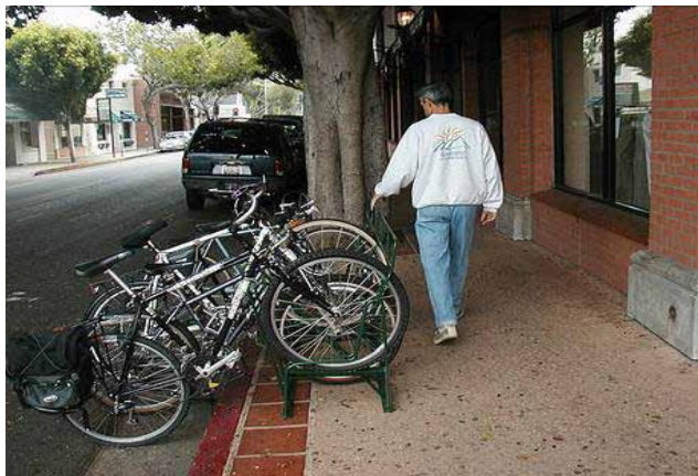
San Luis Obispo, CA uses a combined approach with the bicycle parking sharing sidewalk and onstreet space. This design provides a solution where sidewalk and roadway space is limited.
