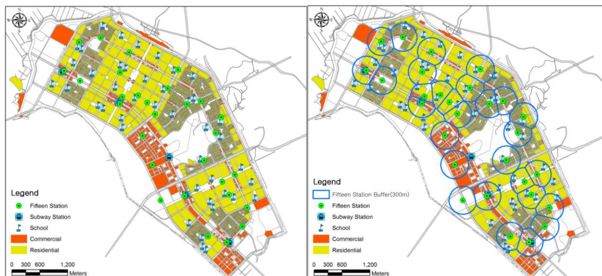
20 21 22 FIGURE 5 Bikesharing Stations in Analysis Site(Ilsan new-city in Goyang)(left) and its Analysis 23 Buffer(right) 24 25
