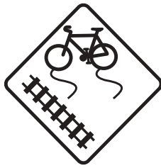
Figure 4-25 Sign warning bicyclists of railroad tracks
