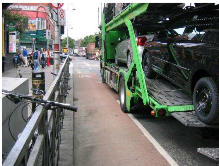
Figure: Pedestrian guardrails may increase the risks to cyclists
