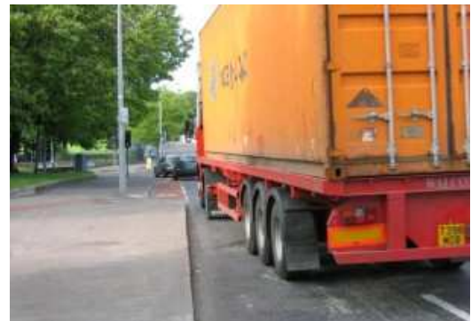
Figure: Cycle lane encouraging cyclists to pass inside left-turning HGVs
