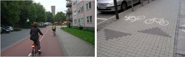
Figure 18. Two-way cycle track with dividing line
