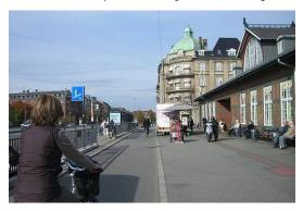
Figure 21. Cycle track passing between bus stop and sidewalk
