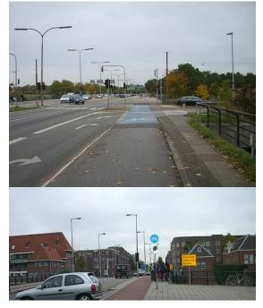
Figure 5. At this unsignallized right turn, the cycle track has dropped to a bike lane with blue coloration and pavement markings through the conflict area.
