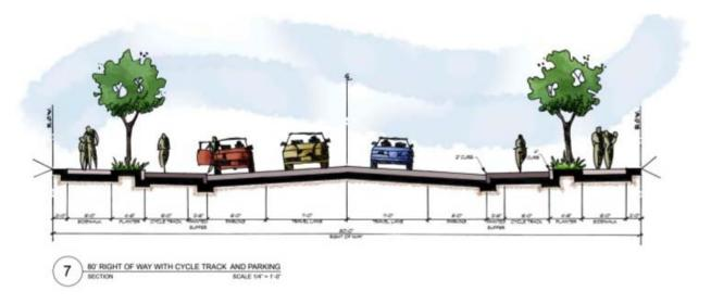
Figure 26. Cross-Section for Cully Boulevard Cycle Track in Portland, OR Source: City of Portland, http://www.portlandonline.com/transportation/index.cfm?c=46784&a=190086
