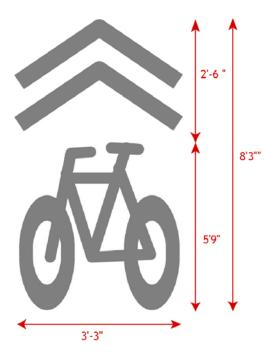
Figure 11. Recommended Modified Bike-and-Chevron
