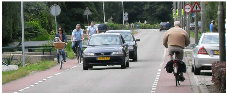
Figure 2: Suggestion lanes on rural and suburban roads in the Netherlands. Notice how the centerline has been obliterated. Cars stay out of the suggestion lane when passing bikes, but enter it when facing oncoming motor traffic.
