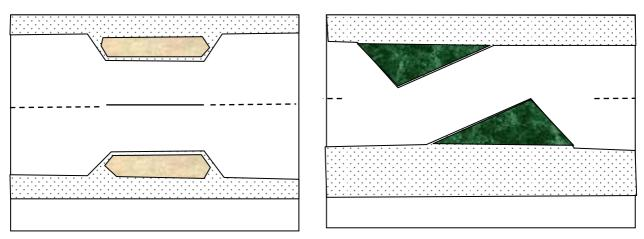
Figure 1: Typical 2-way Pinch-Point and 1-way Chicane
