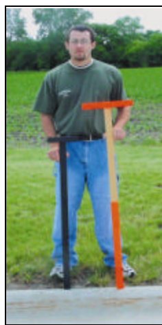
Figure 4.5. Sighting Rod (left) and Target Rod (right)
