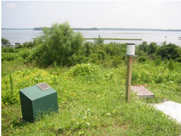
Figure 6. Swansboro monitoring layout from left to right: housing for sampler and bubbler, rain gage, weir box, and runoff spillway.
