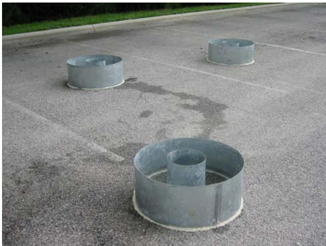
Figure 2. Typical arrangement and setup of double-ring infiltrometers at a site.
