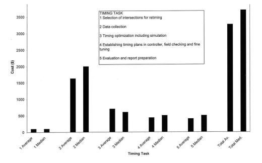
FIGURE 14 Cost for contracted signal retiming tasks.
