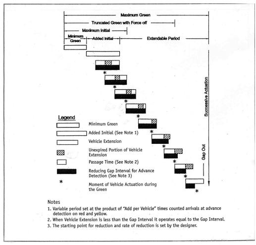
FIGURE 9 Green interval for volume-density operations. (Source: Pline 2001.)
