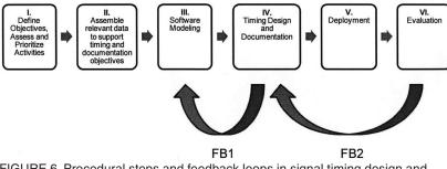
FIGURE 6 Procedural steps and feedback loops in signal timing design and maintenance. (*Source*: Day et al. 2009.)
