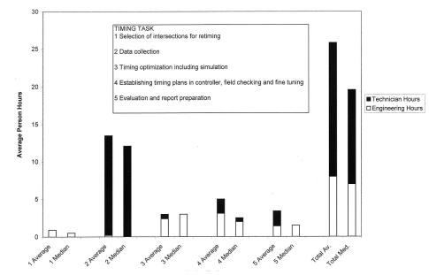
FIGURE 13 Person hours appropriate for signal retiming tasks.
