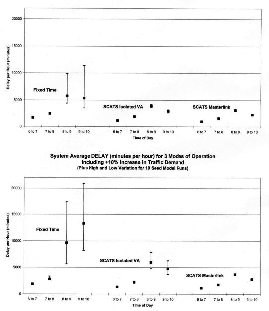
System Average DELAY (minutes per hour) for 3 Modes of Operation (Plus High and Low Variation for 10 Seed Model Runs)
