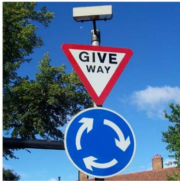
Photograph 3: TSRGD diagram 1003 and TSRGD diagram 611.1
