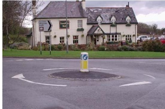
Photograph 5: Street furniture on a domed central island in tarmac creating a small roundabout, not a mini-roundabout
