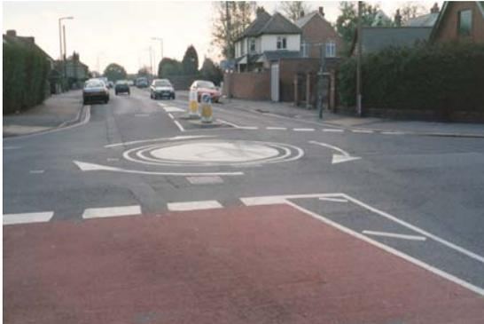
Photograph 4: Non-conforming concentric rings
