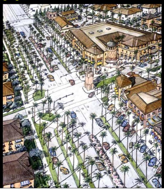
Planning and design concept for restructuring of Palm Canyon Drive as a multiway boulevard to support a downtown on one side of the street (below, with angled parking), housing and lodging on the other (above, with drop-off lane).
