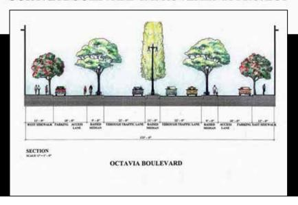
Octavia Boulevard is the first new multiway boulevard built in the United States in 50 years. It was a design voted into place by the community to replace the earthquake-damaged elevated Central Freeway.
