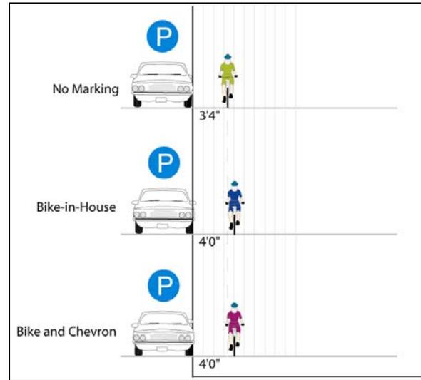
Figure 4. Effect on Bicycle to Parked Car Spacing
