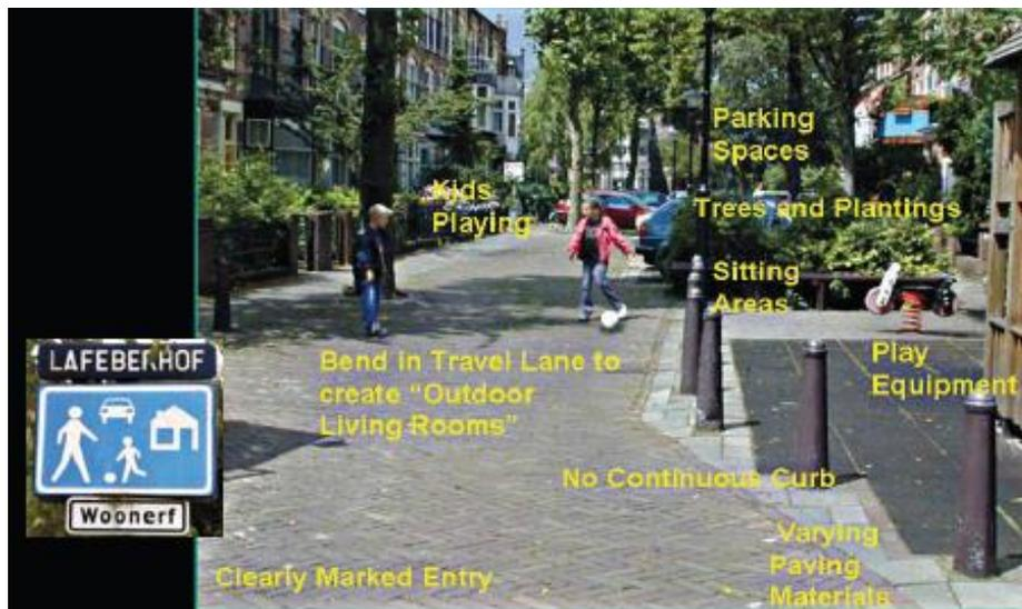
Figure 3: Woonerf design elements | Source: Appleyard and Cox 2006, 31.
